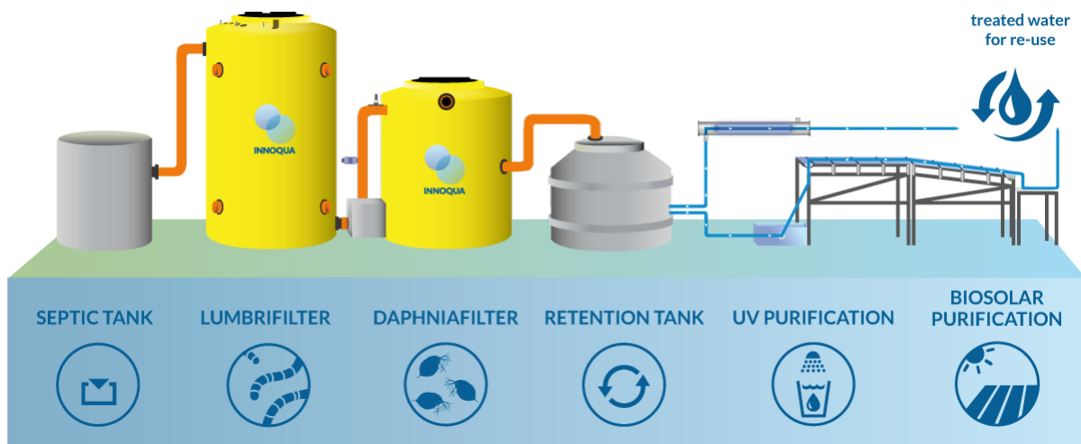
INNOQUA System – Technical Configuration
