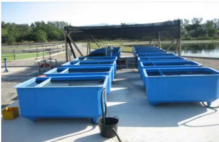
Figure 4-4 Daphniafilter Test Setup at UDG
