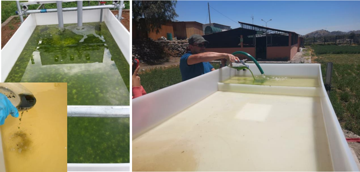
Figure 4-1 BSP inoculation and biofilm formed within 1 week - India (left) and BSP inoculation -Peru (right)
